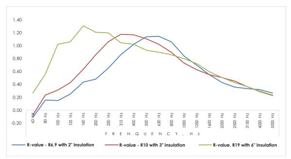
\* Acoustical testing has been performed according to ASTM C423, "Test Method for Sound Absorption and Sound Absorption Coefficients by the Reverberation Room Method".
